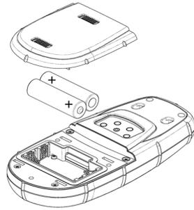
Replace the cover and push the two buttons fully to the right. Verify that the cover is locked in place.
