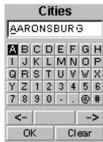
Using the arrow keys to navigate the displayed keyboard, begin typing in the name of the waypoint (destination) you are looking for.
