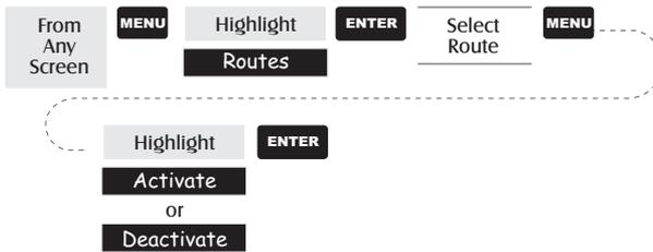
(Note: If the route is active, the Meridian will automatically display “Deactivate Route” in the menu and inversely if the route is not active, “Activate Route” will be displayed.)
