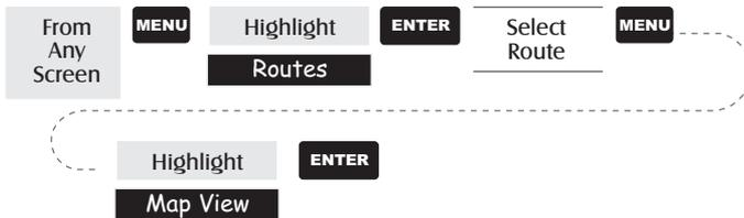
**Editing a Route** — Enables you to modify an existing route by inserting a leg, deleting a leg or replacing a leg. Follow the instructions above for *Viewing a Route* and then use the instructions for inserting, deleting, replacing or appending a leg as appropriate.
