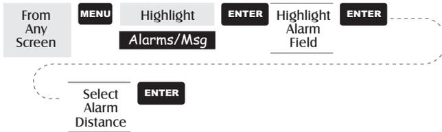
**Setting the Arrival Alarm** — The arrival alarm alerts you that you have arrived at the destination of your GOTO or to the destination of any leg in a route you are navigating on. This option allows you to set the distance from the destination that the alarm will begin to sound.
