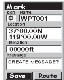
The screenshot shows the 'Mark' screen with the following fields: 'Icon' (a crosshair symbol), 'Name' (WPT001), 'Location' (37°00.00N, 119°00.00W), 'Elevation' (00000ft), and 'Message' (CREATE MESSAGE?). At the bottom, there are two buttons: 'Save' (highlighted) and 'Route'.
